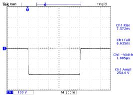
AVO-6C-B-N waveform. 10 kHz, 1 us, -250V into a  $50\Omega$  load (no output module). 100 V/div, 200 ns/div.
