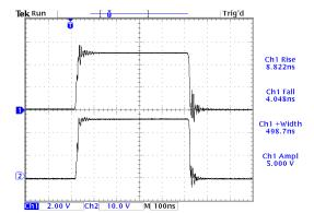
Top: Output of Tektronix CT-2 current probe, measuring an AVO-6C-B-P +5A current pulse through a 1N5819 diode soldered to the output module. 1A/div, 100 ns/div. Bot: MON output, into a  $50\Omega$  load. 10V/div, 100 ns/div.
